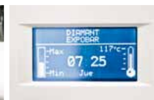
The information display provides valuable data, including the water level in the steam tank
